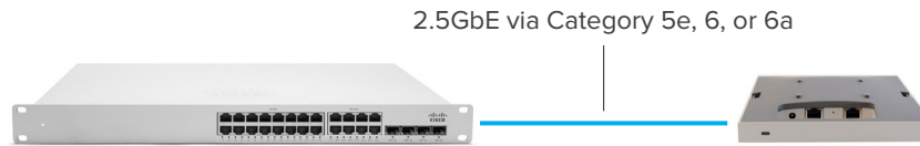
Figure 1 Multigigabit technology can be used with existing cable types and lengths
